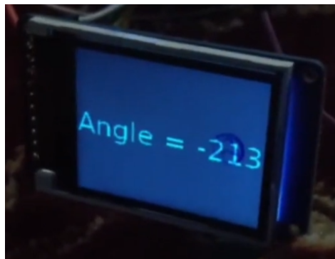
Fig. 14. Screenshot the LCD working and displaying a wrist Angle.
